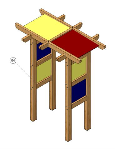
Check the post spacings are the same top and bottom and are square (90°) using a set square. Fill the second trench with post/cement mix and allow to set, following the manufacturers recommended times. Finally, insert the 2 No. 'Beater' into the metal O-Rings located on both panels.
