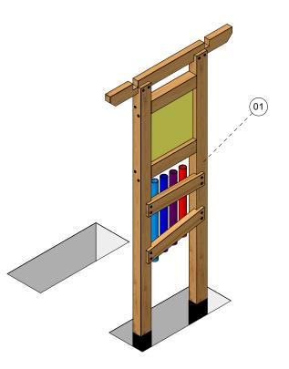
Insert 'Side Panel A' into the holes, ensuring that the music chimes are facing inwards (towards the remaining holes). Check that the frame is level and fill the trench with post/cement mix, following the manufacturers guides.
