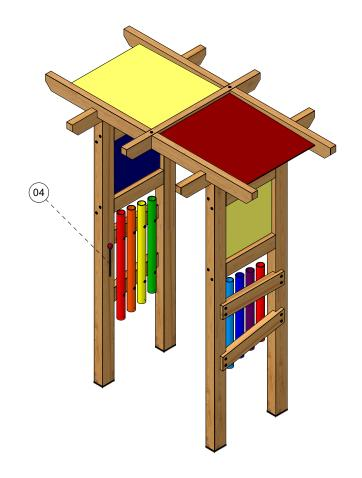
Check the post spacings are the same top and bottom and are square (90°) using a set square. Fill the second trench with post/cement mix and allow to set, following the manufacturers recommended times. Finally, insert the 2 No. 'Beater' into the metal O-Rings located on both panels.
