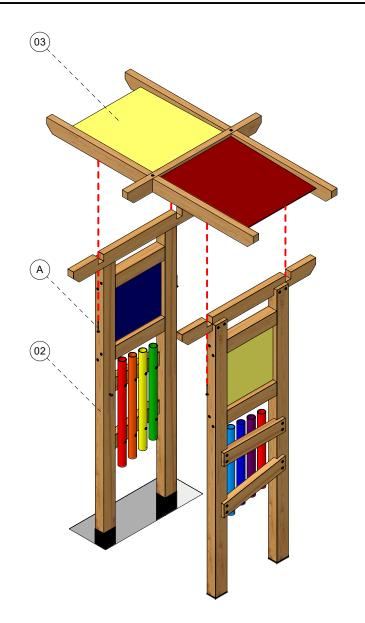
Insert 'Side Panel B' into the trench, ensuring the chimes are facing inwards. Check that the panel is level, then attach 'Roof Panel' to both side panels using the supplied fixings (additional person required to support panel).
